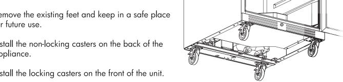
NOTE: Once caster installation is complete, the appliance must be allowed to stand upright for 6 hours before plugging in to avoid damage to internal components.
